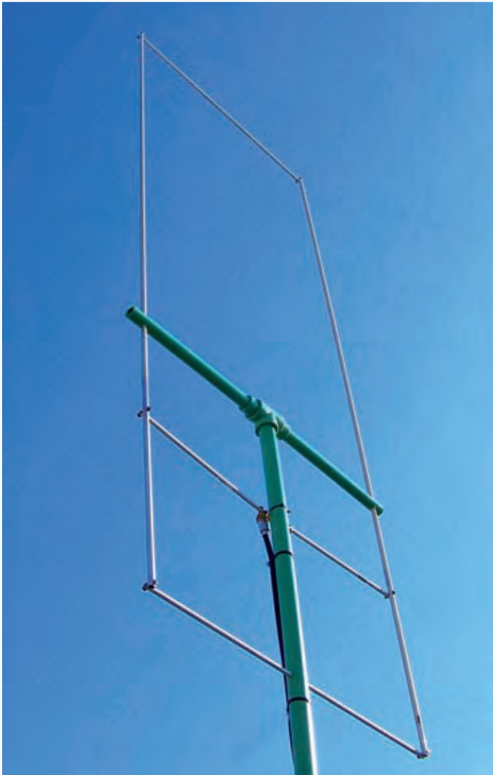
Fig. 3: The Hentenna, constructed by Frank IZ8DWF
